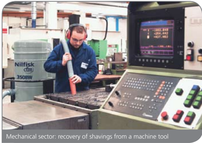
Mechanical sector: recovery of shavings from a machine tool
